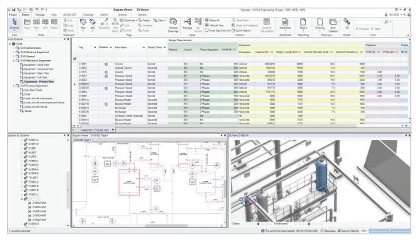
Due to the Integrated IE&D platform, users of AVEVA Engineering can access and reference a comprehensive set of data from other applications as they work. This enables P&IDs and the 3D model to be viewed for the currently focused engineering object.
